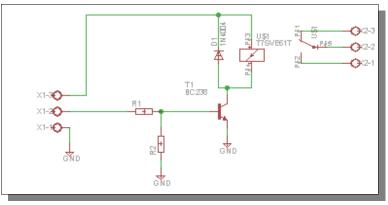
consequently, the relay will be shut down. The diode D1 prevents that extra-voltages generated by the relay, when turned off, could damage the transistor T1.
